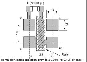
capacitor at a location as near as possible to the power source terminal of the crystal product (between Vcc - GND).
